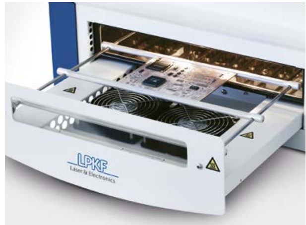
A lit-up process chamber allows for visual inspection during reflow soldering
