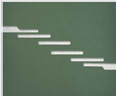
Then processing of large surfaces using milling technology (copper rub-out)
