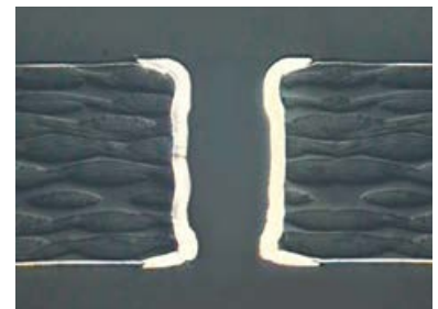
Through-hole plating with LPKF ProConduct
